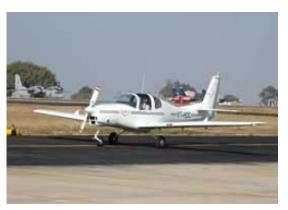
lakh for completion in two-three years. The objective was to build indigenously, a low cost and acceptable cruise efficient aircraft with an all-up-weight of about 500-600 kgs and power around 70-90 bhp<sup>37</sup>. The cost of each aircraft was expected to be less than Rs.5 lakh initially. In November 1993, NAL flew HANSA-2 on experimental basis.
